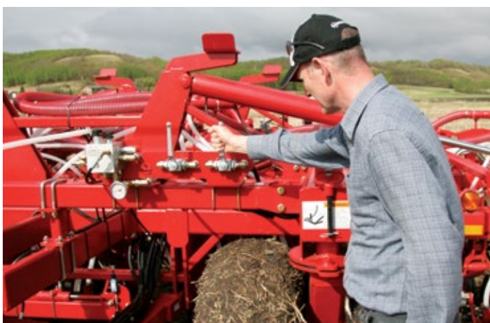
Hydraulic valve manifold for opener pressure
