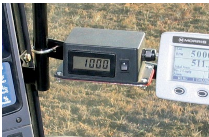
In-cab pressure control
