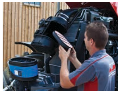
The well proportioned cooling package is easy to access, clean and maintain. 90% of dust is removed naturally thanks to the suction from the cooling fan.
