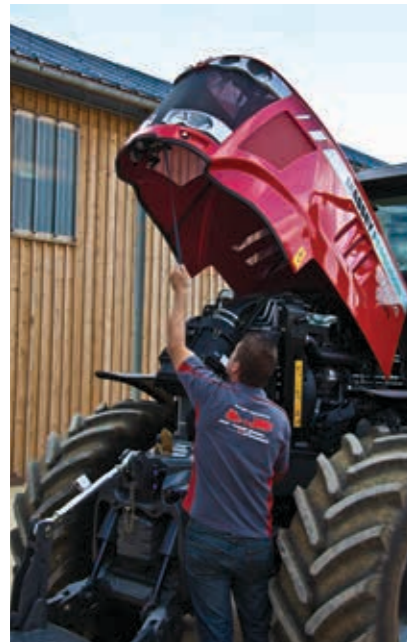
The single piece bonnet lifts fully to allow excellent access for full servicing
