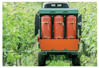
3 different type of gas containers: "EU", "US"and "US small". Gas tank frames and the amount of containers are developed for extended operating time.
