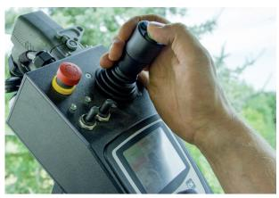
Easy Access to all relevant functions: C-CONTROL PREMIUM steerage with touchscreen display and joystick.
