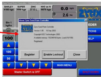
The software version number and date on this screen will change in the event of a software upgrade. It is important that this information is recorded in this Operator's Manual to keep track of any changes.
