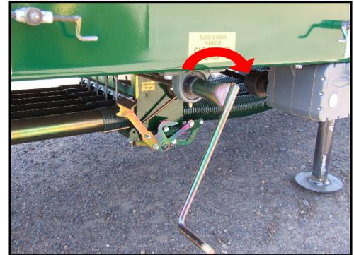
**Step 9.** Record the weight of the product metered and enter into the Simplicity Zynx X20 Console as per the Variable Seed Rate Control Operators Manual. The 'Calibration Factor', which is the relationship between the calibration shaft turns and the weight of the product metered, is then automatically calculated.
