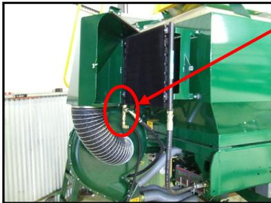
The oil cooler is protected by a relief valve which is pressure set in the factory to divert oil in the case of a pressure build up. A pressure build up is commonly caused by a restriction in the hydraulic return line usually being a quick release coupling being uncoupled.
