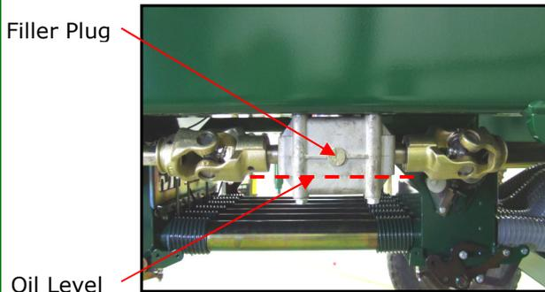
The oil level in each 'T' Box should be checked at the start of the sowing season.
