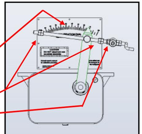
**Step 6.** Rotate the calibration handle clockwise until product flows from the metering unit freely and evenly. This will prime the metering unit with product and allow for accurate calibration.
