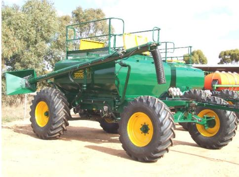
Load/Unload auger in the stowed position
