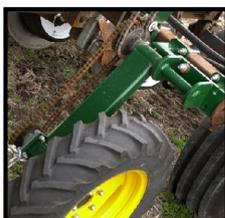
"Drop Wheel" drive consists of an independent wheel contacting the ground to provide drive via a chain to the Air Seeder. With a "Drop Wheel" drive it is advisable to avoid cornering with the wheel on the ground so as to avoid any lateral pull on the wheel.
