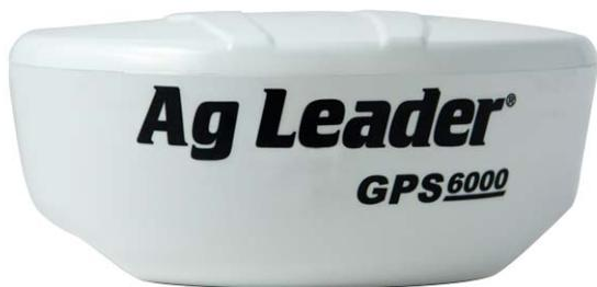
The GPS 6000 is a high-performance GNSS receiver and antenna, capable of receiving and tracking different combinations of GPS L1 and GLONASS L1 code and carrier signals on a maximum of 14 channels. SBAS (Satellite Based Augmentation Systems) support, which includes WAAS, EGNOS, and MSAS, is standard. The GPS 6000 rear panel also features light emitting diodes (LEDs) for status indication.
