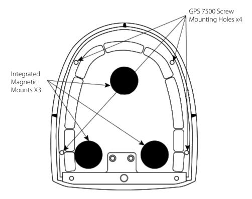
The GPS 7500 must be mounted with the connector facing the side of the vehicle.
