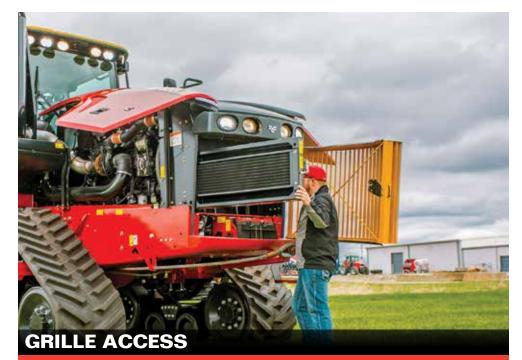
The front grille swings open to provide ground level service access to the condenser / cooler package.
