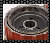
The DeltaTrack was designed using the legendary Versatile outboard planetary system. In addition to doing a better job of putting power to the ground the outboard planetary is far easier to service than competitive inboard units. Removing the planetary cover exposes the planetary gears and sun gear for easy access.
