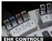
Electro-hydraulics are available in a four-valve set up and an optional six-valve cofiguration.
