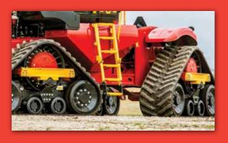
A right hand ladder gives you access to the engine air cleaner for quick servicing. The ladder also helps with right side fueling and provides access to the egress door and folds up and out of the way when not in use.
