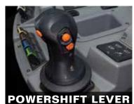
A four-function powershift lever gives you quick control over forward, reverse, upshift and downshift functions, eliminating the need for a clutch pedal.
