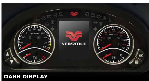
A programmable center high-resolution display provides readouts on; transmission functions, engine functions, field monitoring and basic tractor functions. RPM, speed, temperature and fuel are all displayed on simple to read analog gauges.
