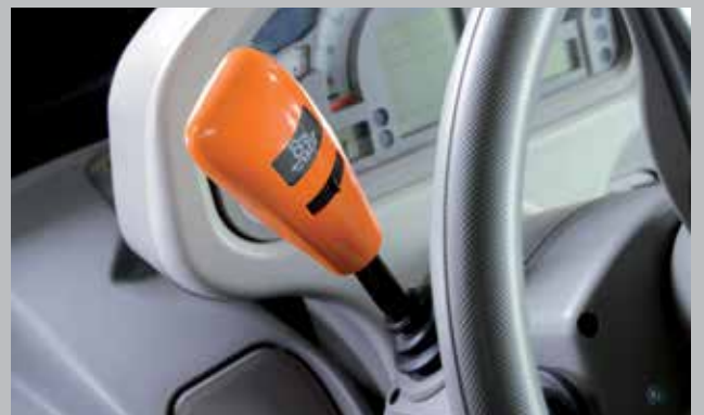
Powershuttle as standard. Electro-hydraulic reverse shuttle with adjustable five stage settings
