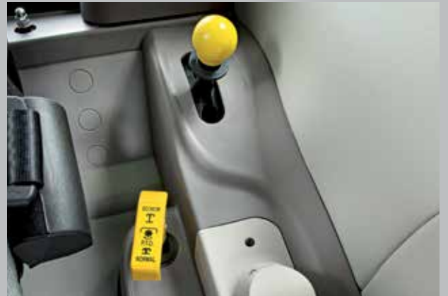
PTO speed selector lever with the selection of 4 speeds.
