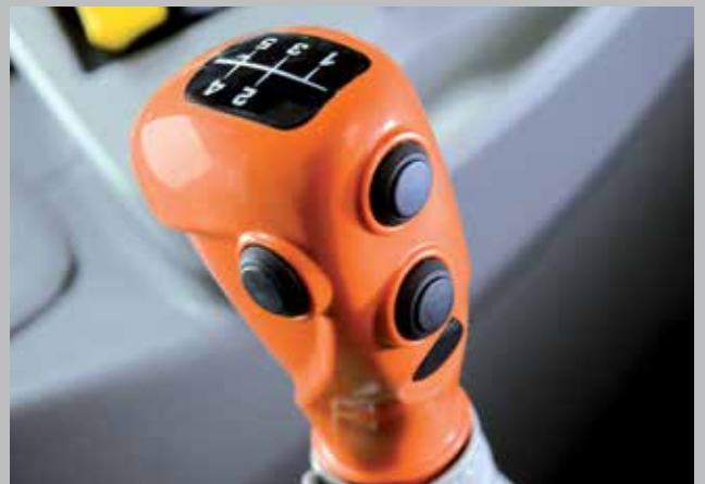
Bowden cables have made gear changing even more convenient at the push of a button.
