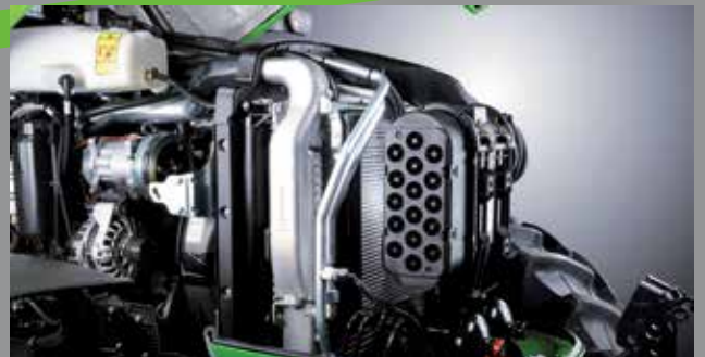
... as does the easy-to-clean cooling system with its viscous fan (optional).
