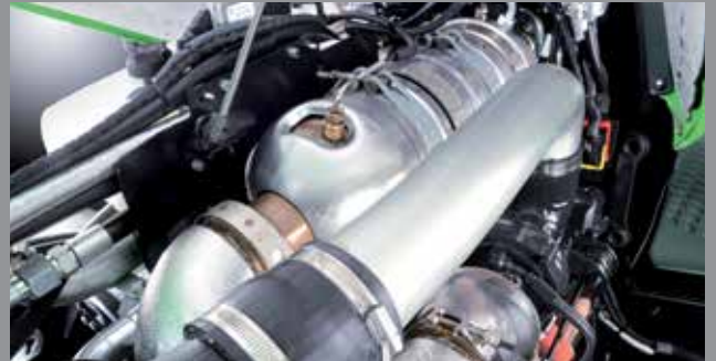
Diesel oxidation catalyst (DOC) catalytic converter guarantee minimum emissions.
