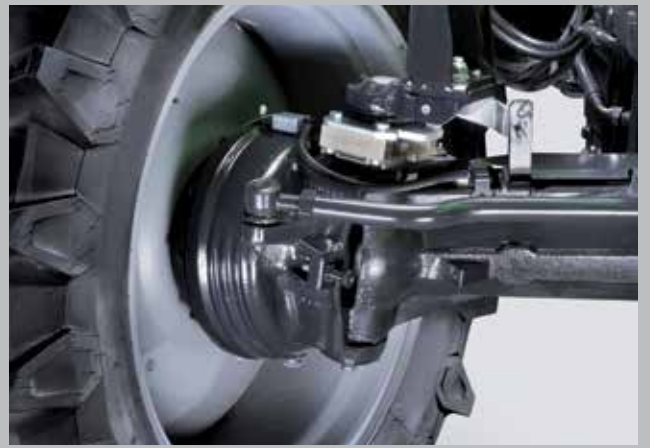
A unique safety concept from DEUTZ-FAHR. Separate oil cooled disc brakes on the front wheels.
