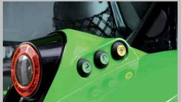
External PTO and rear lift controls for straightforward equipment mounting and external PTO operation.
