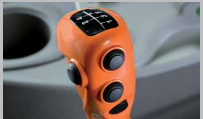
Comfort clutch and Powershift. Simply change gear at the push of a button without pressing the clutch pedal.
